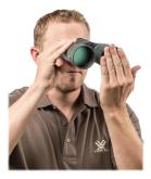
on the right eyepiece) toward your eye to unlock and adjust. Rotate the diopter until the object is in focus. Then, push the diopter ring back down to lock your settings. Make note of this diopter setting in case you need to set it again. From this point on, you will only need to use the center focus wheel.
