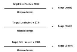
Using either the vertical or horizontal mrad scale, place the reticle on the target of known dimension and read the number of mrads spanned. Obtain maximum accuracy in ranging by calculating exact mrad measurements—try to estimate mrad measurement in 1/10s if possible.
