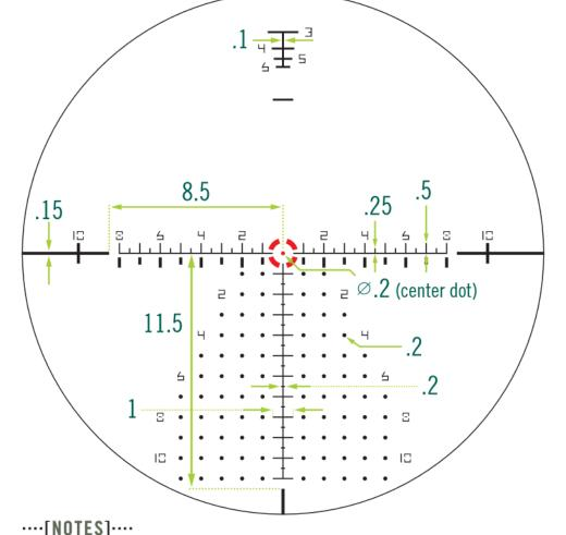
Subtensions are measured in MRAD and remain constant at all magnifications. Ø=Diameter
