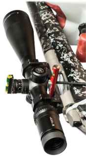
Using bubble levels to square the rifle scope to the base.
