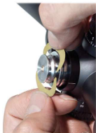
Alternate shim installation direction with each shim.
