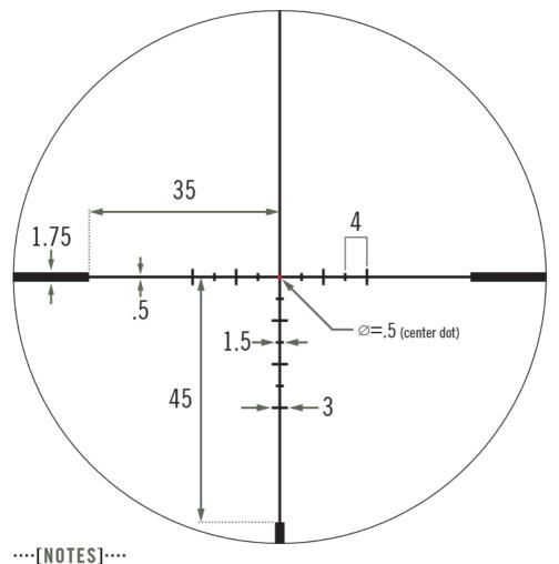
Subtensions are measured in MOA and correspond to the highest magnification. Ø=Diameter
