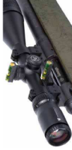
Use of bubble levels to square the riflescope (and reticle) to the base.
