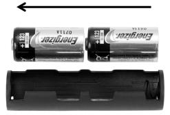
Load two CR-123 Lithium batteries with the positive terminals pointing in the direction of the arrow. NOTE: The flashlight cannot be charged with the CR-123 CARRIERm installed.
